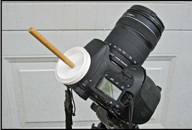
Figure 2: "PolaSun™" polarization finder mounted on hot shoe of DSLR camera.
